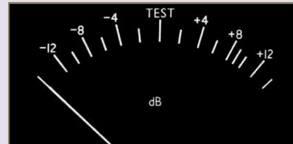
EBU PPM scale – also in 4dB steps "Test" is usually set for -18dBFS
