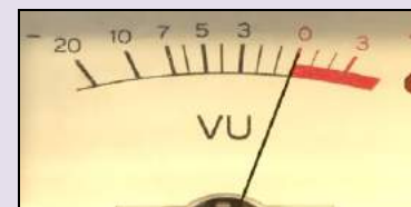
Just right (0VU = 18dB below clip) Noise-free without clipping
