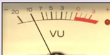
Too low (-10VU = 28dB below clip) Wasting dynamic range
