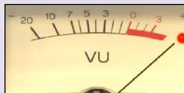
Too high Peaks could be heavily clipped
