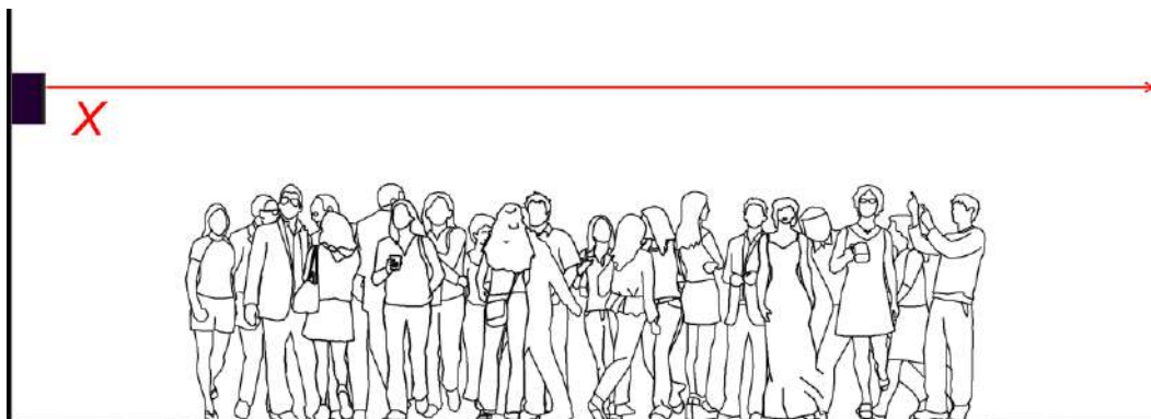
Fig 6.2-1 Poor vertical aiming
