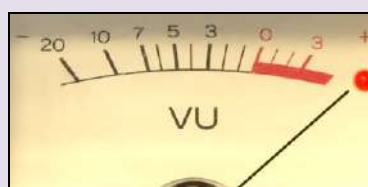
Too high Peaks could be heavily clipped
