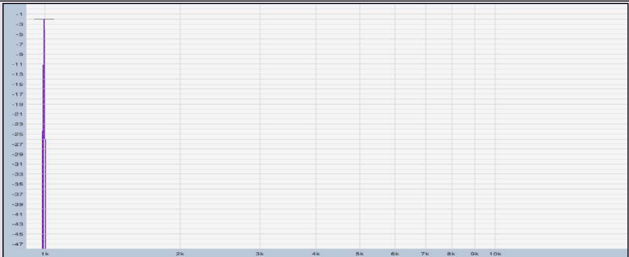
1kHz pure tone just below clip level (Vertical = level in decibels, horizontal = frequency)
